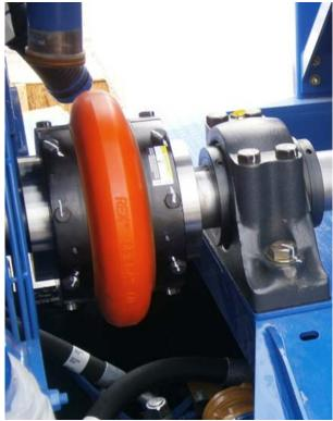
Figure 14: Flexible coupling installed
