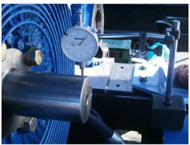
Figure 4: Dial indicator on stub shaft
